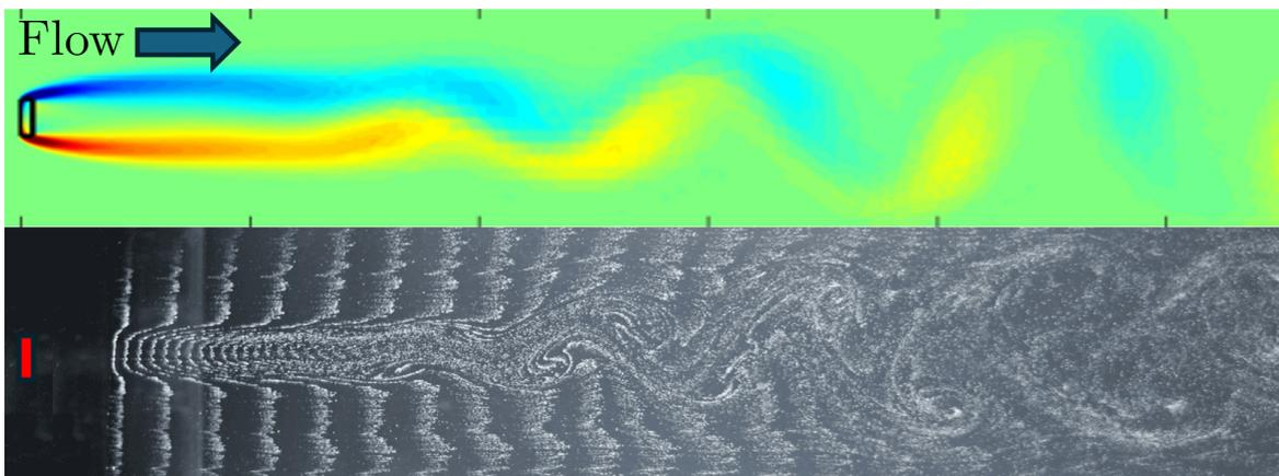
**Figure 1:** *The 2D flow around a highly permeable rectangle: numerics (on the top) and visualization with hydrogen bubbles (on the bottom) of the wake. Downstream of the object, a steady shear layer develops and destabilizes at a large distance from the body, with the formation of a von Karman vortex street.*
